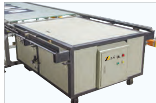
摆渡台 Ferry Station
